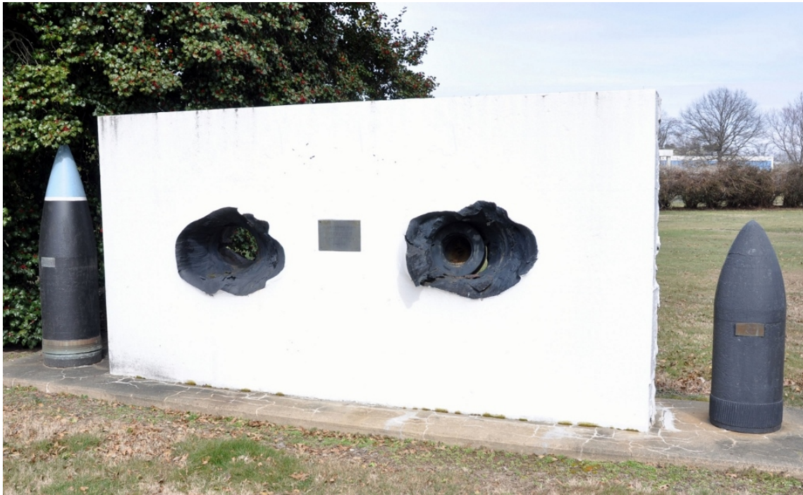
Figure 1 - USS Alabama (BB-60) Armor Test Plate. Photograph courtesy of NSWC, Dahlgren.
